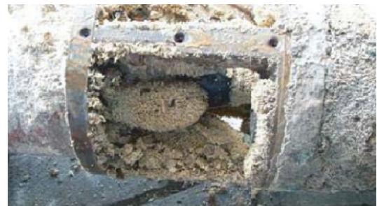
Sea life growth inside the pump intake and on the pump shaft
