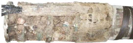
Sea life growth covering the pump bowls and intake screen
