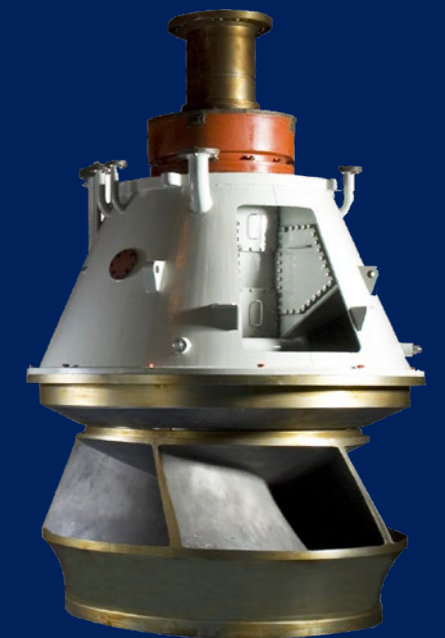
Concrete volute cooling water pump
